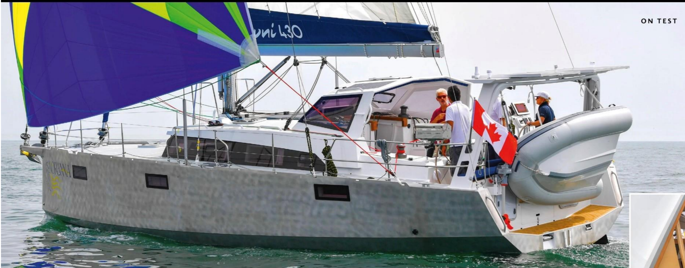
A highly protected cockpit. Note the davits built into the stern arch with a Highfield aluminium rib on the test boat, plus a shallow companionway
