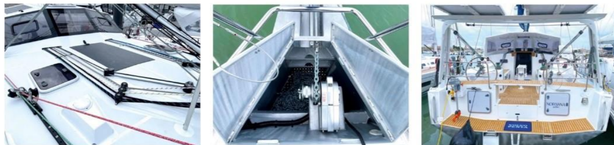
Expansive foredeck is emphasised by full bow sections and a wide sprit that can take two anchors, while the sugarscoop and arch add more useful space
